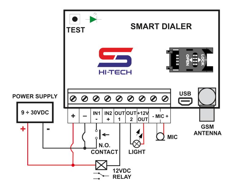
A suitable place for module's installation in lifts is behind the cabin's button panel with adhesive tape. The emergency push button and the LED indicator can be mount on the front panel. There must be enough free space in front of the microphone and the speaker for better acoustics.
