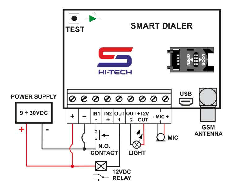
This module can be install behind the cabin's button panel with adhesive tape. The emergency push button and LED indicator have to install at the front panel. There must be free space in front of the microphone and the speaker for better acoustics.
