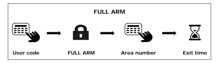
Arming will start by counting the exit time with audible signal (short beeps) and flashing the ARM status indicator in red. In the last few seconds, the beeps will speed up. Exit time will end with the ARM tone - three consecutive beeps, where the last is longer and the ARM status indicator lights steadily red.
